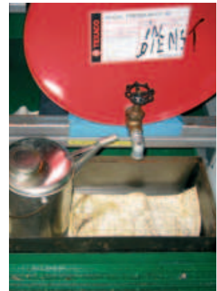
OP pads under oil cans & drums to catch small drips.
