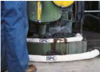
Solution: SOCs quickly soak up leaks and drips for a clean and safe workplace.
